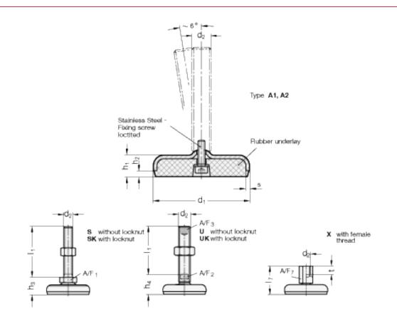
$\begin{array}{l} A/F1 = 17 \\ d1 &= 100 \\ d2 &= M10 \\ h1 &= 20 \\ h2 &= 6 \\ h3 &= 28 \\ l1 &= 80 \\ s &= 3 \end{array}$
